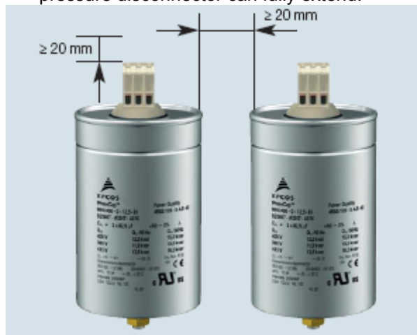
Figure 4: Minimum space over and between the capacitors.
