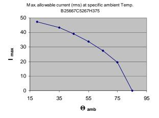
Max. allowable ambient Temp. at specific current (rms) B25667C5267H375
