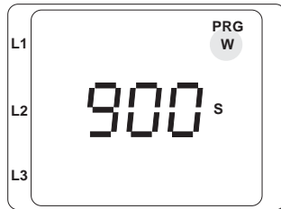
Example for the averaging time of real power mean value, here 900 seconds.
