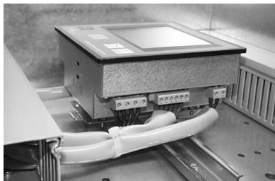
Diagr. Cable connections for UMG 505 UMG505 for DIN rail mounting.
