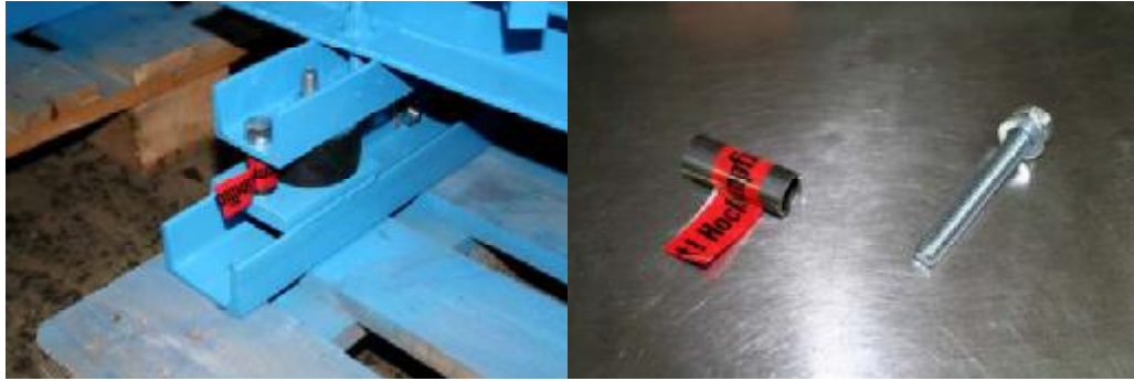
Figure 8: Rubber mounting pad with transportation safety device
