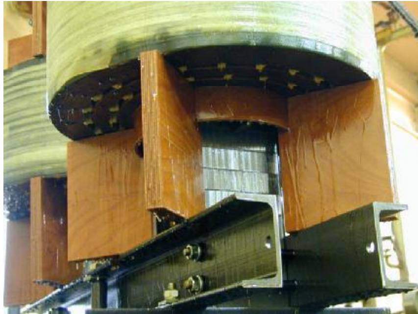
Figure 1: Insulation resin beads on product
