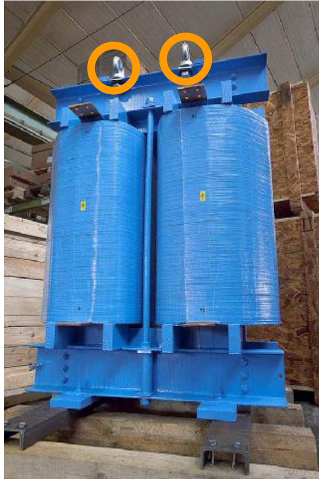
Figure 5: Example for lifting bolts at product
